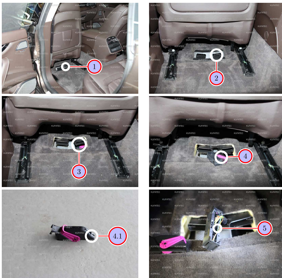
Figure 4: Removing trim panel Quattroporte / Ghilbli from model year 2016 forward - pictures
